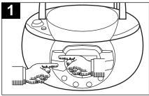
After you insert the disc into the CD player and the total number of tracks appear on the display, you may press either the Skip/Search FWD. (►►) or REV. (◄◄) button to select a specific track for playback.
